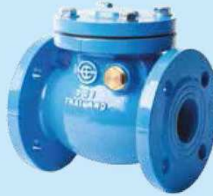
Fig 360 Metal Seated Swing Check Valve AWWA C508 BS 5153 PN 6, 10, 16, 25 BS EN 12334 PN 6, 10, 16, 25 MSS - SP-71 class 125, 150 TIS 383 PN 6, 10, 16 DN 50-1800 (2"-72")
