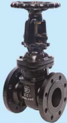
Fig 110 Gate Valve Rising Stem BS 5150 PN 6, 10, 16 BS EN 1171 PN 6, 10, 16 MSS - SP-70 class 125 TIS 432 PN 6, 10, 16 DN 50-300 (2"-12")
