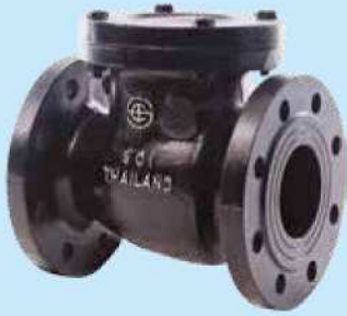
Fig 300 Resilient Seated Swing Check Valve BS 5153 PN 6, 10, 16 BS EN 12334 PN 6, 10, 16 MSS - SP-71 class 125 TIS 383 PN 6, 10, 16 DN 50-300 (2"-12")
