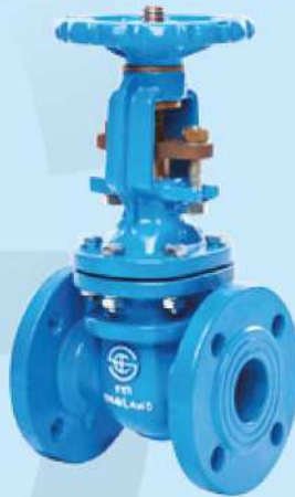
Fig 269 Gate Valve Rising Stem AWWA C500 BS 5150 PN 6, 10, 16, 25 BS 5163 PN 6, 10, 16, 25 DIN 3352 PN 6, 10, 16, 25 TIS 256 PN 6, 10, 16 DN 50-300 (2"-12")
