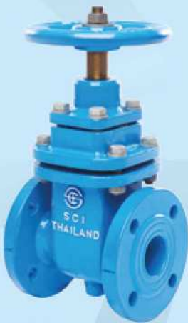
Fig 131 Gate Valve Non Rising Stem AWWA C500 BS 5150 PN 6, 10, 16, 25 BS 5163 PN 6, 10, 16, 25 DIN 3352 PN 6, 10, 16, 25 TIS 256 PN 6, 10, 16 DN 50-600 (2"-24")
