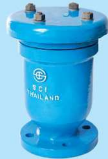
Fig 430 High Speed Air Valve JIS B 2063 PN 7.5, 10, 16 TIS 1368 PN 10, 16, 25 DN 50-300 (2"-12")
