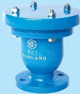
Fig 413 Single Large Orifice Air Valve JIS B 2063 PN 7.5, 10, 16 TIS 1368 PN 10, 16, 25 DN 50-150 (2"-6")
