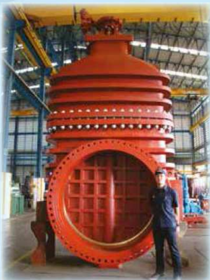
Fig 131 Gate Valve Non Rising Stem AWWA C500 BS 5150 PN 6, 10, 16, 25 BS 5163 PN 6, 10, 16, 25 DIN 3352 PN 6, 10, 16, 25 TIS 256 PN 6, 10, 16 DN 50-600 (2"-24")
