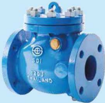
Fig 300 Resilient Seated Swing Check Valve BS 5153 PN 6, 10, 16 BS EN 12334 PN 6, 10, 16 MSS - SP-71 class 125 TIS 383 PN 6, 10, 16 DN 50-300 (2"-12")
