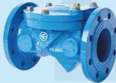
Fig 383 Rubber Flapper Check Valve Non Slam Performance BS 5153 PN 10, 16 BS EN 12334 PN 10, 16 MSS-SP-71 class 125 DN 50-600 (2"-24")
