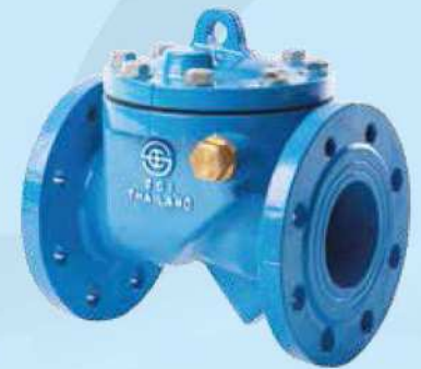
Fig 483 Tilting Disc Swing Check Valve BS 5153 PN 6, 10, 16 BS EN 12334 PN 6, 10, 16 MSS-SP-71 class 125 DN 80-1800 (3"-72")
